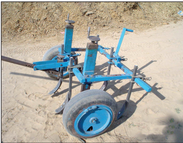
Fig 2. Pneumatic wheeled multipurpose tool frame with cultivator arrangement.
